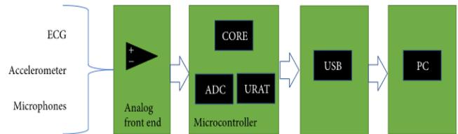
Fig. 1. Block diagram of audio acquisition system [6].
