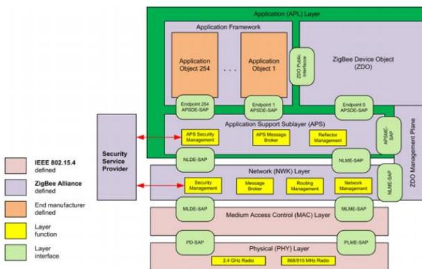
Fig. 2. Zigbee protocol architecture [10]
