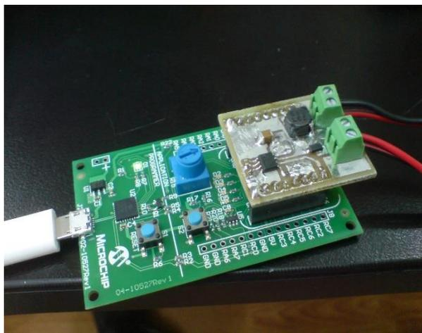
Fig. 2. The MPLAB Xpress board with the converter power circuit on top.
