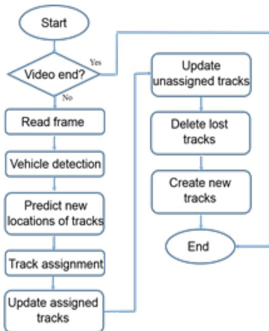
Fig. 2. The flow chart of vehicles tracking method
