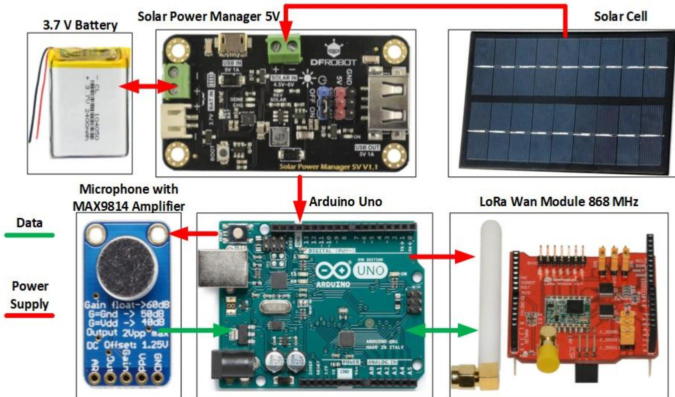
Fig. 2. Block diagram of a process information point.
