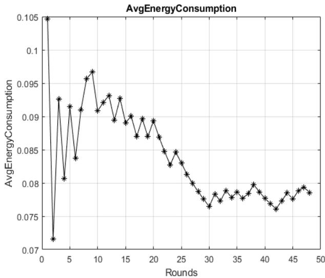
**Figure 4.** Example of energy consumption from a wireless sensor network, with different number of transmitted data packets
