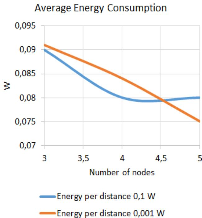
**Figure 5.** Average energy consumption of a wireless sensor network
